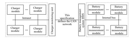
Fig. 2. Station network physical architecture of electric vehicle charging
