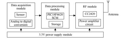
Fig. 4. Station network heterogeneous hierarchical data fusion diagram of electric vehicle charging based on Tiny0S
